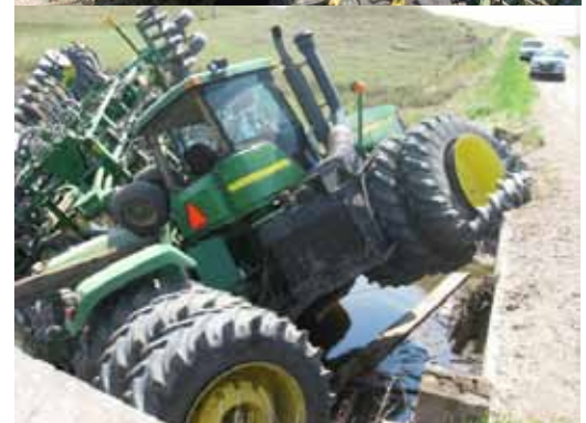
THE TRACTOR LOST POWER AS IT WAS CLIMBING THE HILL. IT THAN PROCEEDED TO ROLL BACKWARDS DOWN THE HILL, CONTROL WAS LOST AND IT ENDED UP IN THE CREEK.
